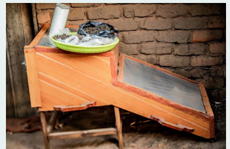
A solar dryer that is used by the caregroups to dry and remove moisture content in food substances ©UNICEF/2023/HD Plus
